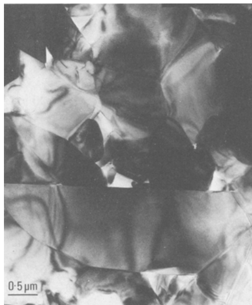
Figure 7 Transmission electron micrograph showing the microstructure of a hot-pressed Zr–O–F ceramic ( F/Zr = 0.16 , 30 min at 800^\circ\text{C} , 22.5 MPa, \rho = 5.50\text{ g cm}^{-3} ).
